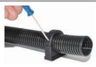
To remove the conduit insert a small screwdriver where it states OPEN. Push down and lever to release. The hinge should then be free to open.
